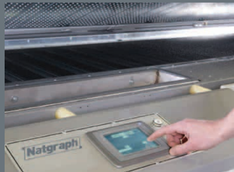
Touch Screen PLC Control
